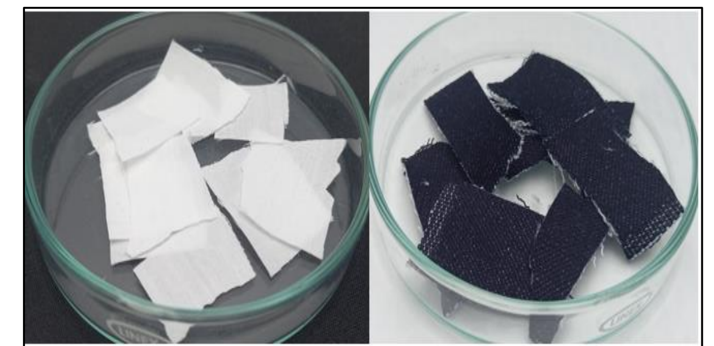
Figure 1. Pictures of the original materials. From left to right: PCS (75% PES/23% CO/2% EL) and SQUASH POPLIN (84% CO/14% PES/2% EL)
