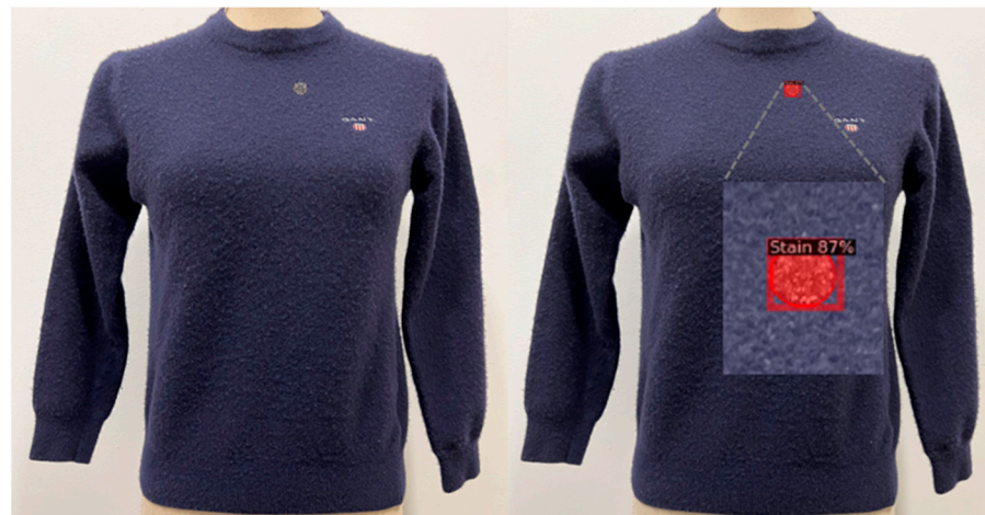
Figure 7. Stain detection with the corresponding class label, bounding box and pixel-level identification.
