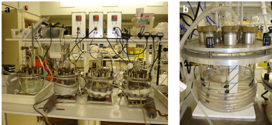
Figure 3.1 Photograph of the two stage chemostats installation (a) and a vessel with the coupons (b).
