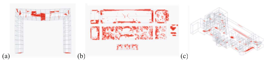
Fig. 13. Maximum principal strains: a) stone frame with node P4; b) vaults (bottom view); c) masonry walls (same color scale).
