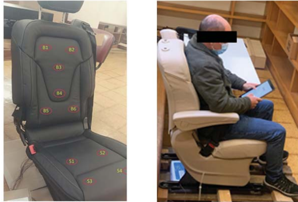
Fig. 1. Seat with the locations where the vibration actuators were installed (on the left), and the final setup (on the right).
