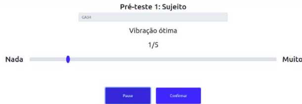
Fig. 5. Graphical user interface developed for the vibration intensities evaluation.
