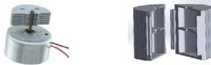
Fig. 2. The motor from Vybronic, model JQ24-35F580C (on the left), and the 3D printed shield used to prevent contact with the eccentric mass.
