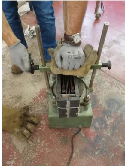
Figure 73 - Moulding Box placement for aluminium cast.
