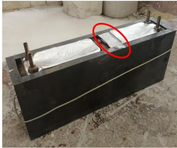
Figure 75 - Problems found after the casting.
