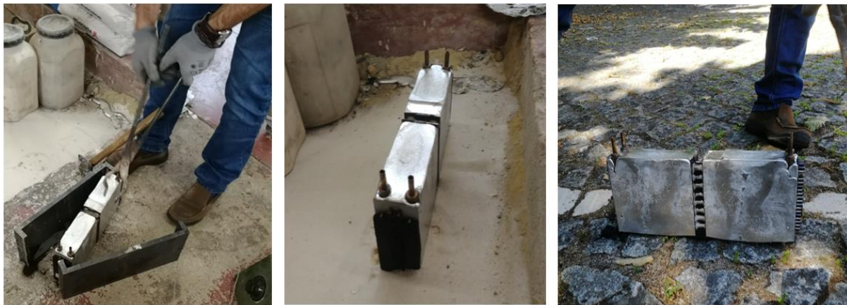
Figure 76 - (a) Moulding Box extraction and cooling (b) inside and (c) outside.
