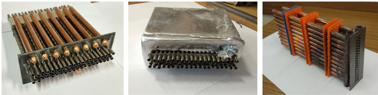
Figure 28 - a) HPs and corrugated pipes placement planning; (b) Corrugated pipes casting tests and (c) 3D printed Positioners prototypes.
