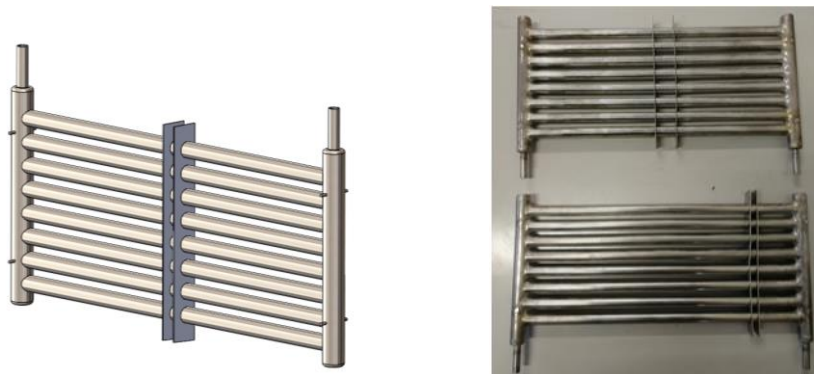
Figure 64 - (a) CAD model and (b) built stainless-steel Heat Pipes.
