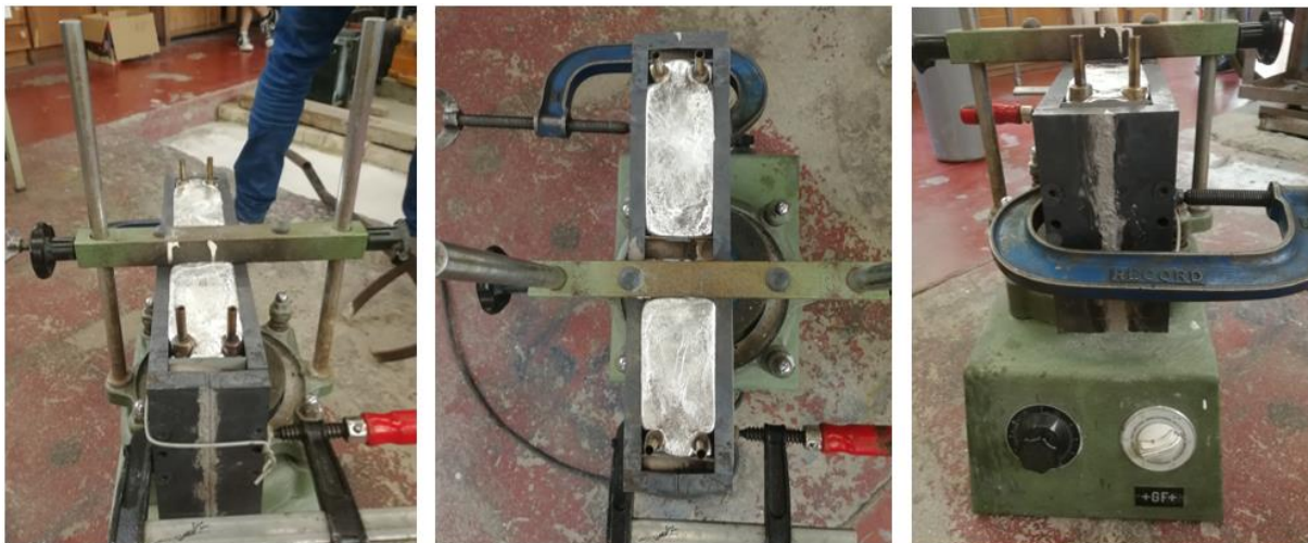
Figure 74 - (a), (c) side-view and (b) top-view of the moulding box after aluminium casting
