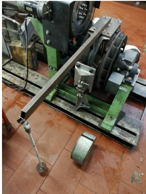
Figure 97 - Dynamometric Brake Calibration Procedure.
