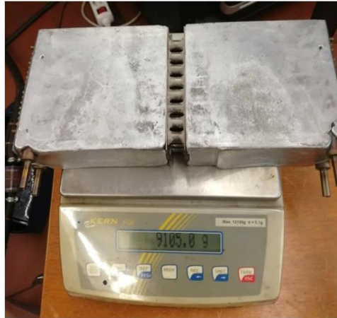
Figure 79 - Weighted TCTG after casting
