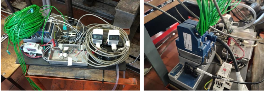
Figure 41 - (a) Data acquisition system table and (b) NI CompactDAQ modular system in blue.
