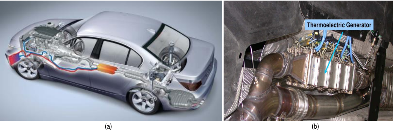
Figure 22 – (a), (b) TEG Installed in a BMW 530i [82] [83].
