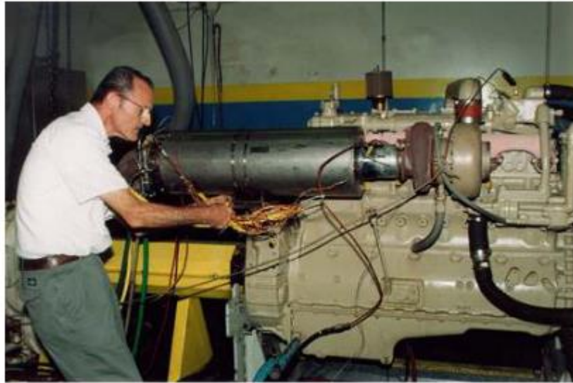
Figure 17 - 1 kW Generator Mounted on Cummins NTC350 Engine [70].
