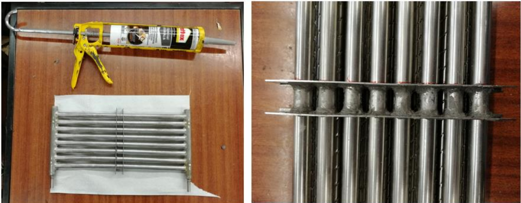
Figure 68 - (a) high temperature silicone and (b) after application on positioners.
