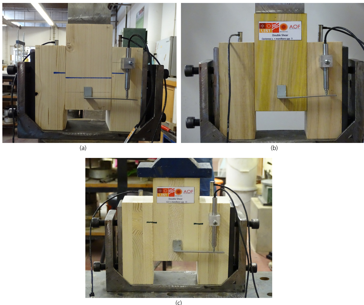
Figure 6. Set-up of the double-shear tests performed to evaluate the performance of the wooden dowels: (a) spruce; (b) chestnut and (c) CLT made of spruce
