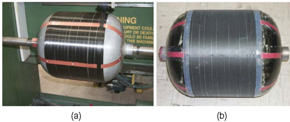
Fig. 6. (a) SMART Layer strips embedded on bottle during filament winding process; (b) finished bottle. Adapted from [54].
