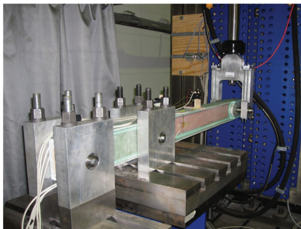
Figure 26. Sub-component (beam) during a cyclic loading. [284]
