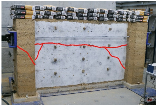
Fig. 2. Crack pattern of URE-IP model.
