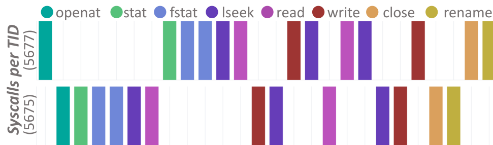
Figure 5.4. Syscalls issued over time by RansomEXX's encryption threads to file F10573.bqt.vmdk.
