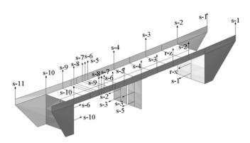
Figure 12 – Layout of measuring points for the dynamic tests in Övik Bridge.
