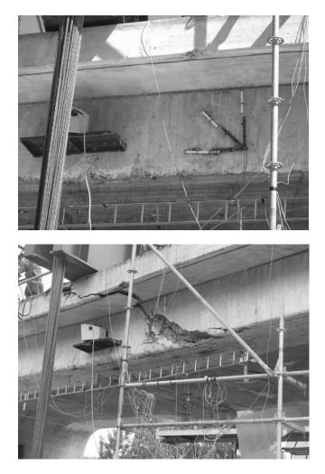
Figure 11 - Cracking in the lateral beam; (top) first damage test; (bottom) final failure test.
