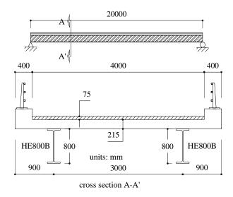
Figure 2 - Geometry of the composite bridge adopted as example.
