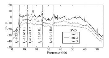
Figure 16 – Singular Values of the Spectral Density Function for all setups in the final damage test.
