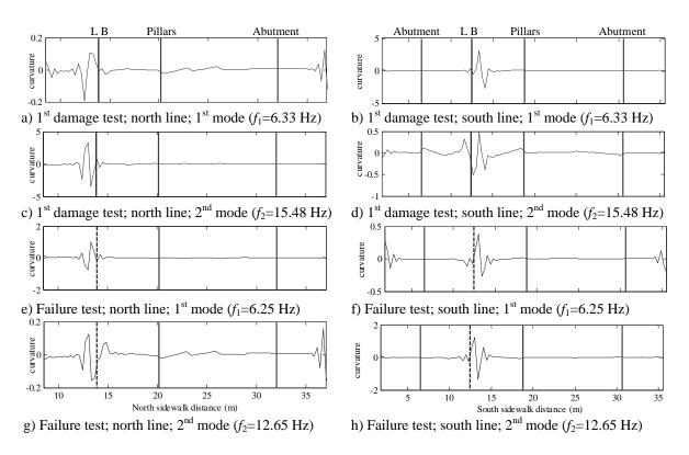
Figure 18 - Curvature method applied to the first two mode shapes in the deck of the bridge.
