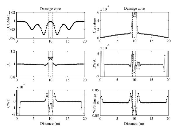
Figure 6 - Typical comparison of level 2 damage detection methods (crack depth I4 and crack location D2, noise not added).
