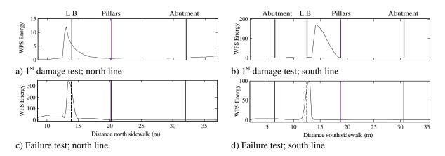
Figure 21 - WPS applied to the acceleration along the deck of the bridge.
