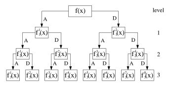
Figure 1 - Wavelet Packet Transform at 3rd level of Decomposition.
