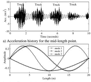
b) Three first mode shapes for the undamaged case
