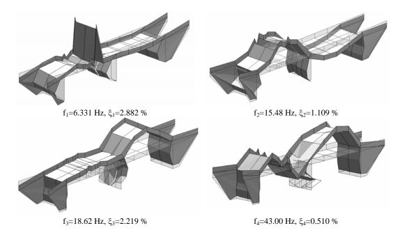
Figure 15 - Estimated mode shapes for the first damage test.
