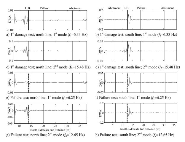
Figure 19 -DWA method applied to the first two mode shapes in the deck of the bridge.
