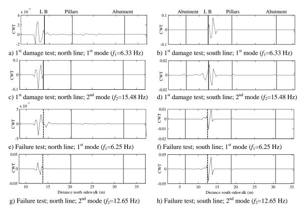
Figure 20 - CWT method applied to the first two mode shapes in the deck of the bridge.
