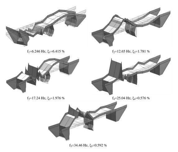
Figure 17 - Estimated modal parameters for the final failure test.
