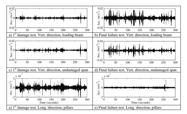
Figure 13 – Comparison of the acceleration histories in some location in the bridge.
