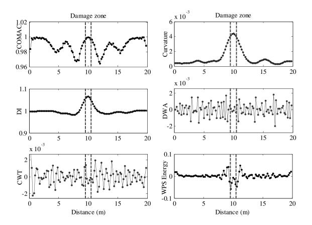
Figure 7 - Typical comparison of level 2 damage detection methods (crack depth I4 and crack location D2, noise level 1.0%).
