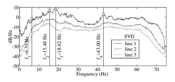
Figure 14 – Singular Values of the Spectral Density Function for all setups in the first damage test.
