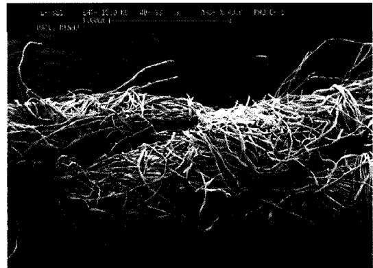
Fig. 46. Electron microscope picture of the 295.00 g/km yarn.
