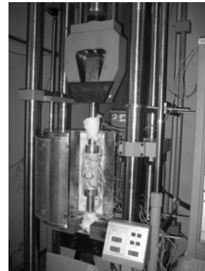
Figure 1 Compression tests at high temperatures
