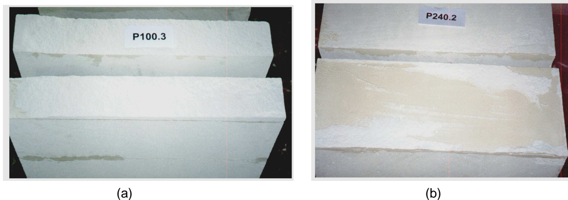
Figure 13 – Aspects of the failure surface for different height of the wall: (a) 100 mm and (b) 240 mm
