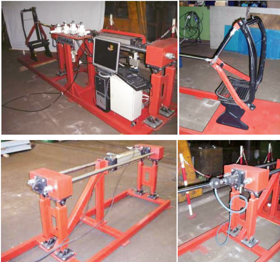
Figure 5. Views of the actual dynamic test system of car seat deformations.
