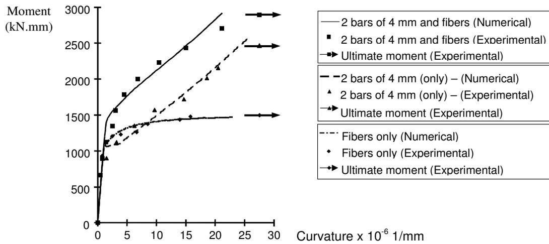
FIG. 9. Numerical versus experimental (Kormeling *et al.* 1980) moment-curvature relationship
