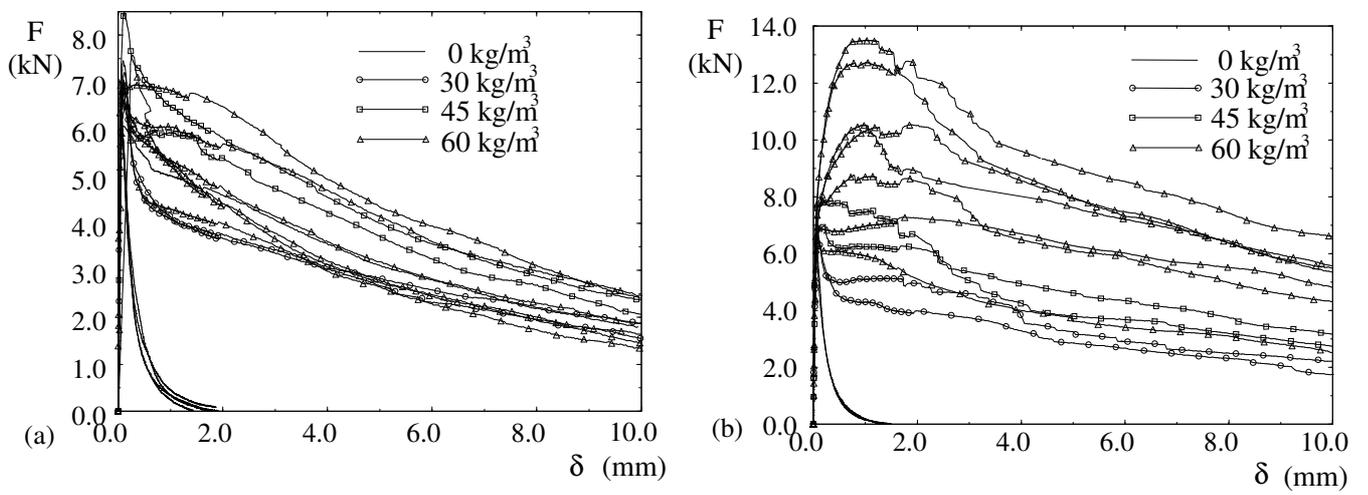
FIG. 4. Load-displacement relationship obtained in three-point bending tests of the notched beams of series *s3* (a) and *s4* (b)
