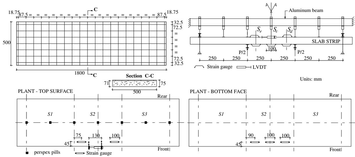
FIG. 10. Slab strip geometry, supports and load arrangement and details of instrumentation
