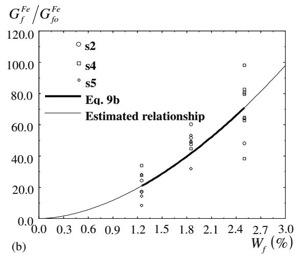
FIG. 5.  $G_f^{Fe} / G_{fo}^{Fe} - W_f$  relationship for specimens reinforced with ZP30/.50 (a) and ZX60/.80 (b) of fibers
