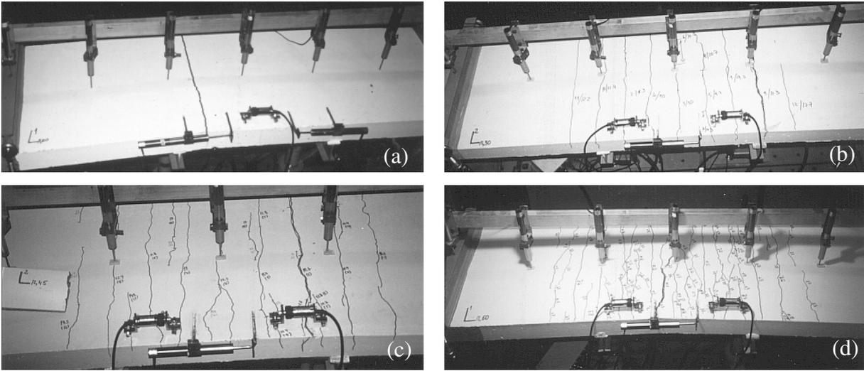
FIG. 11. Typical crack patterns of the slab strips reinforced with wire mesh and 0 (a), 30 (b), 45 (c) and 60 (d)  $\text{kg/m}^3$  of fibers ZX60/.80
