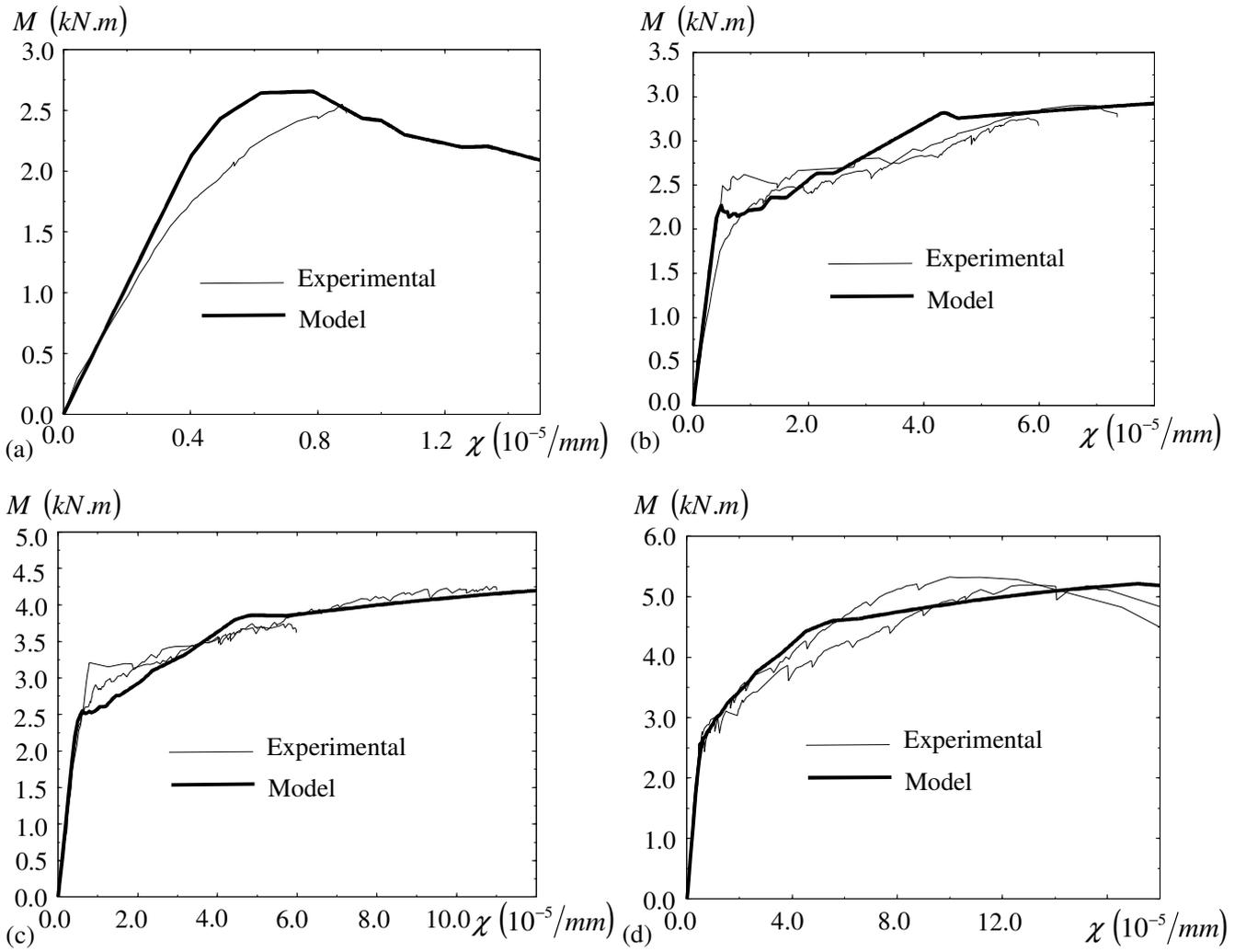
FIG. 13. Moment-curvature relationship of slab strips reinforced with 0 (a), 30 (b), 45 (c) and 60 (d)  $kg/m^3$  of fibers.
