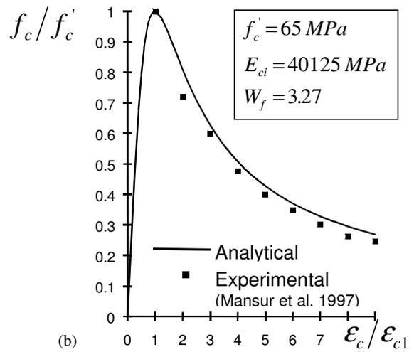
FIG. 2. Analytical versus experimental compression normalized stress-strain relationship for fibers 30/50 and with aspect-ratio of 60
