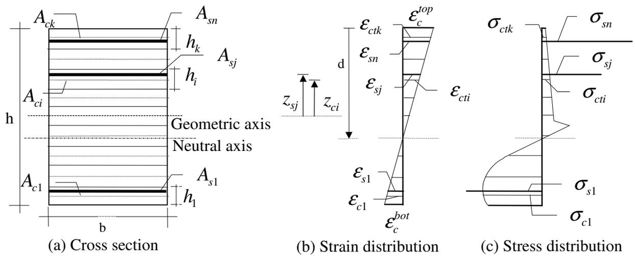
FIG. 7. Cross section discretization and assumed strain and stress diagrams
