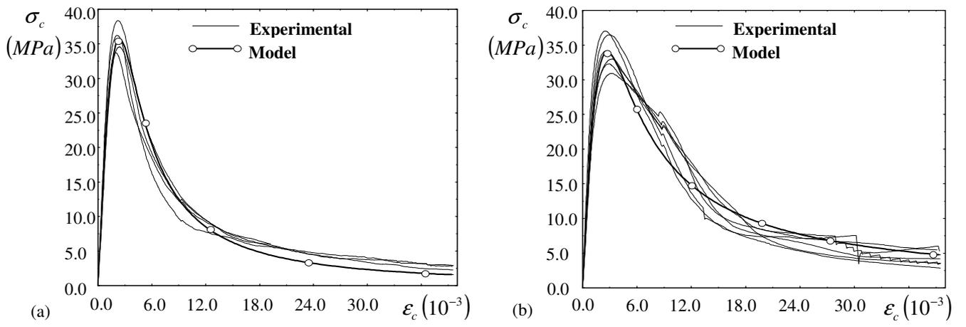
FIG. 1. Analytical versus experimental compression stress-strain curves for series *s4* with 30 kg/m<sup>3</sup> (a) and 60 kg/m<sup>3</sup> (b) of fibers
