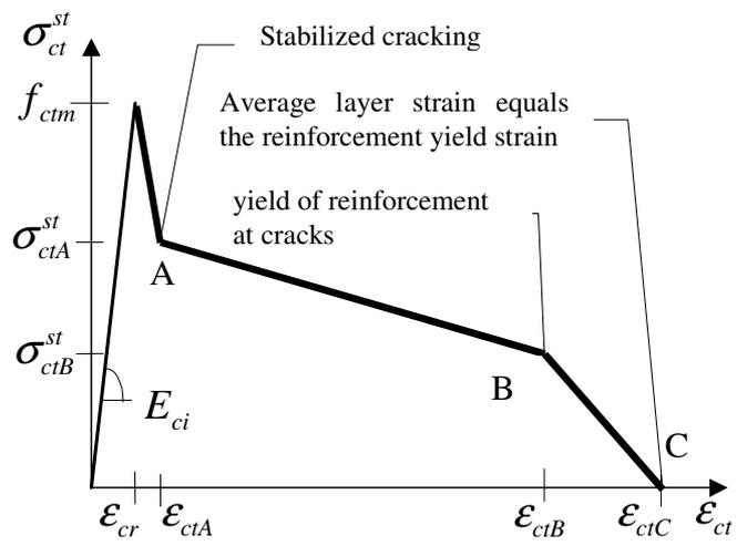
FIG. 8. Tension stiffening diagram
