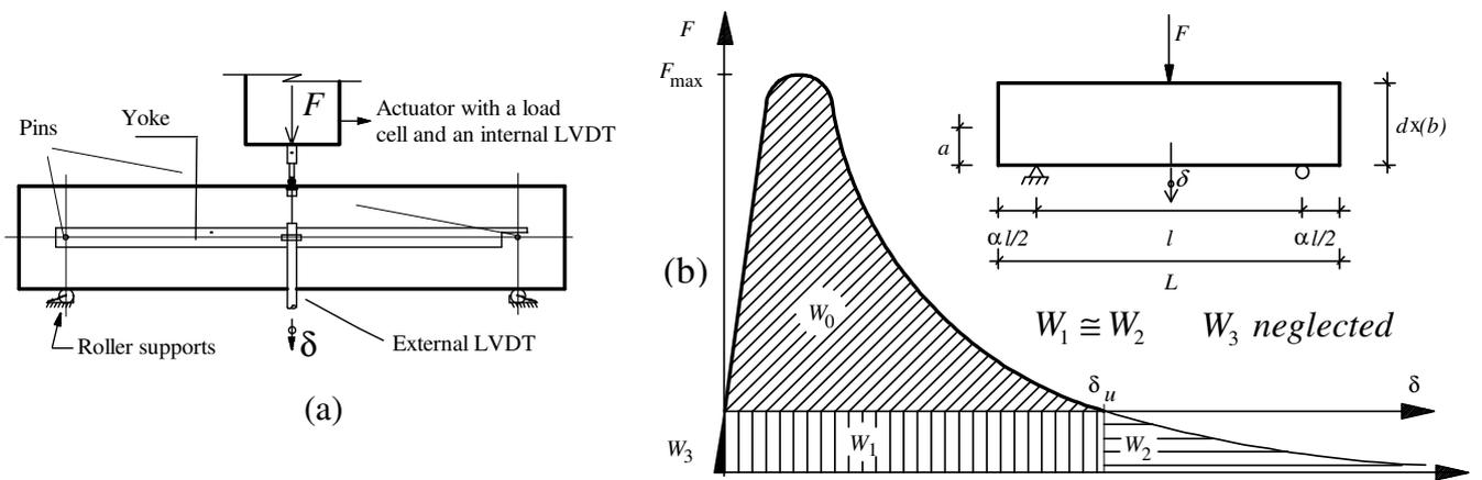
FIG. 3. Setup of flexural test on notched beam (a) and schematic representation of fracture energy evaluation (b)
