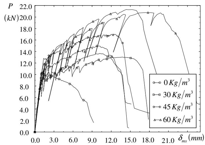
FIG. 12. Relationship between load and displacement at midspan, for the slab strips reinforced with wire mesh and different percentages of steel fibers ZX60/.80
