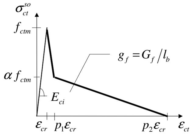
FIG. 6. Parameters used to define the tensile stress strain diagram
