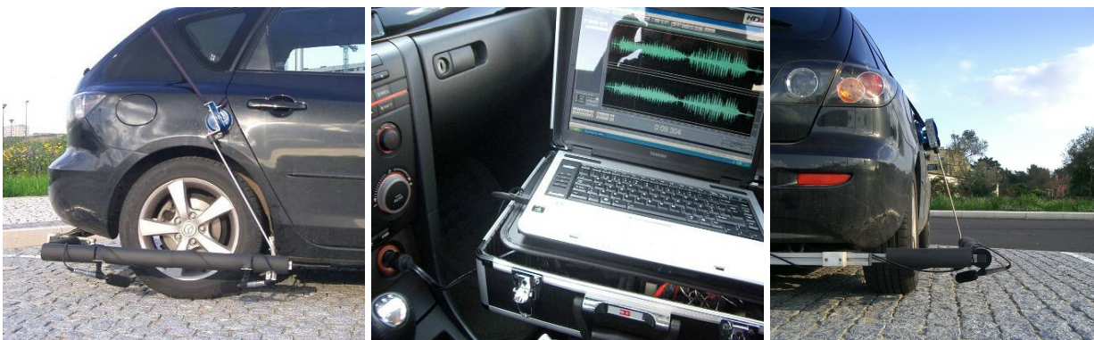
Figure 1 – Close proximity system used for the CPX tests
