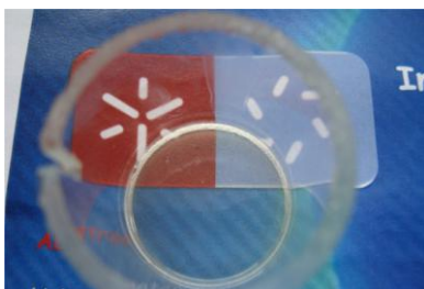
Figure 1- Polymer electrolyte film obtained with composition (a\text{-pEO}_{15\%}/\text{pTMC}_{85\%})_{12} LiTFSI.
