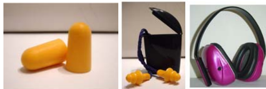
Figure 1 – HPDs used in the test: moldable earplug, pre-molded earplug and earmuff.
