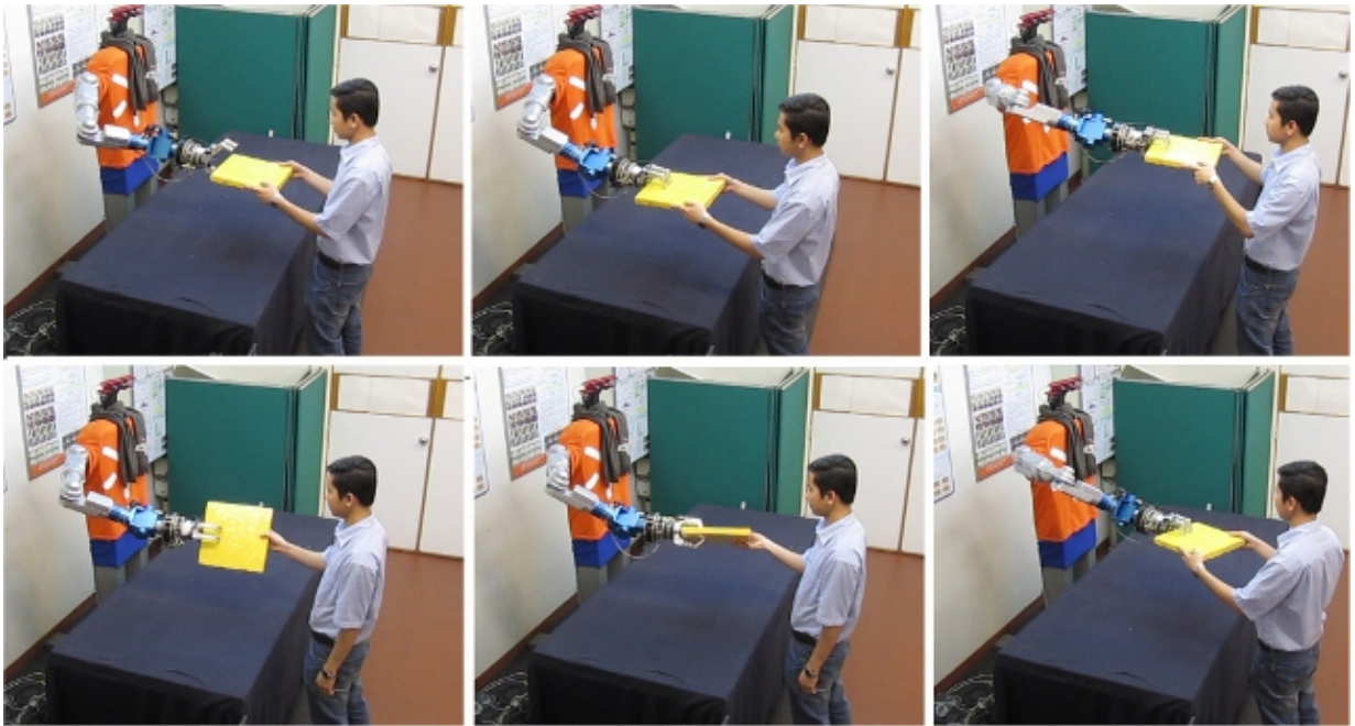
Figure 5.6: The robot ARoS reacts sensitively to forces, torques interactions from a human (Video 4).
