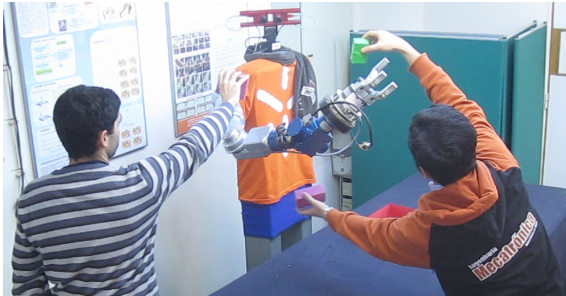
Figure 4.1: An application of tracking and grasping a mobile object in a dynamic obstacle environment with the experimental Anthropomorphic Robotic System - ARoS
