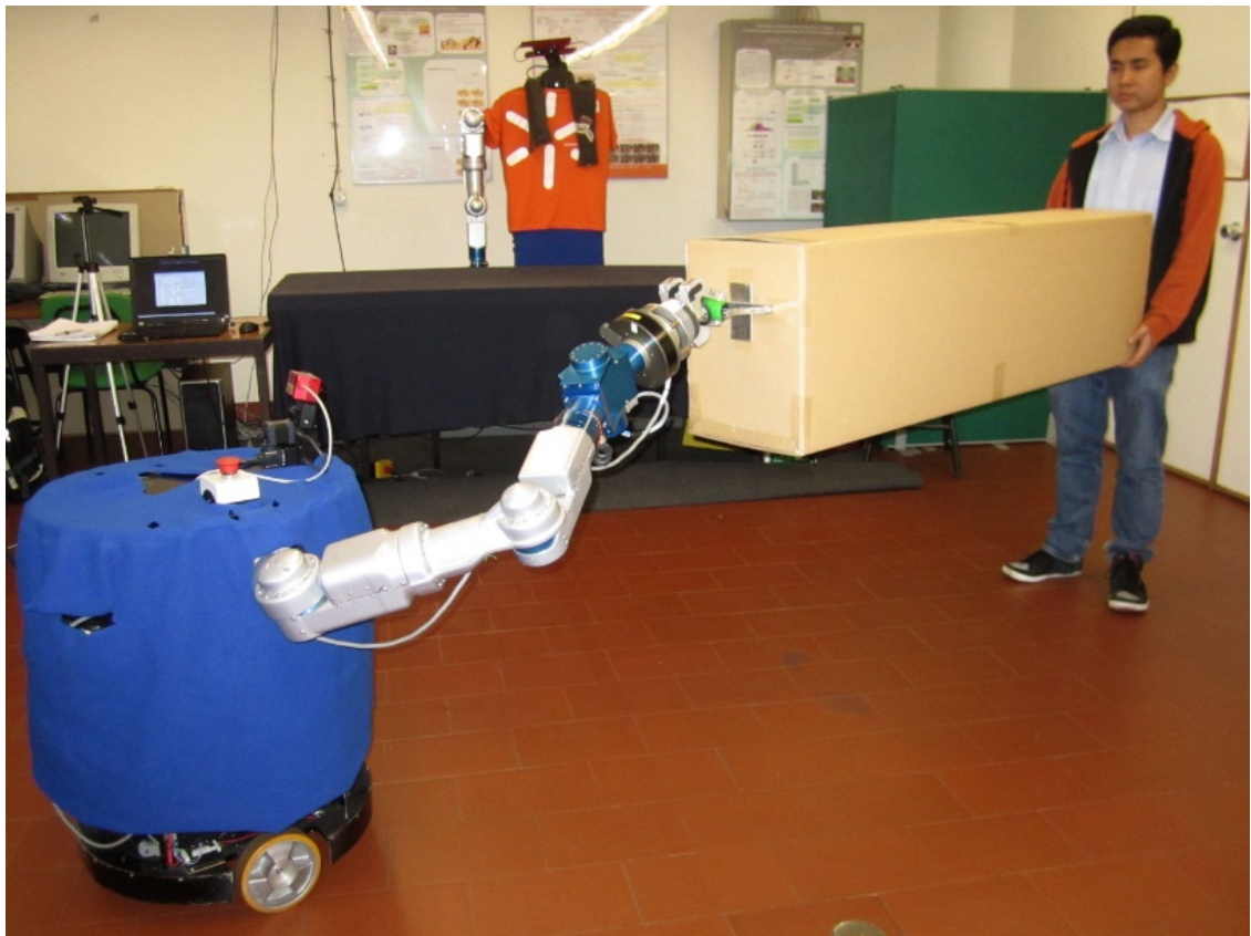
Figure 6.1: Dumbo, an anthropomorphic mobile manipulator, is performing a cooperative object transportation task
