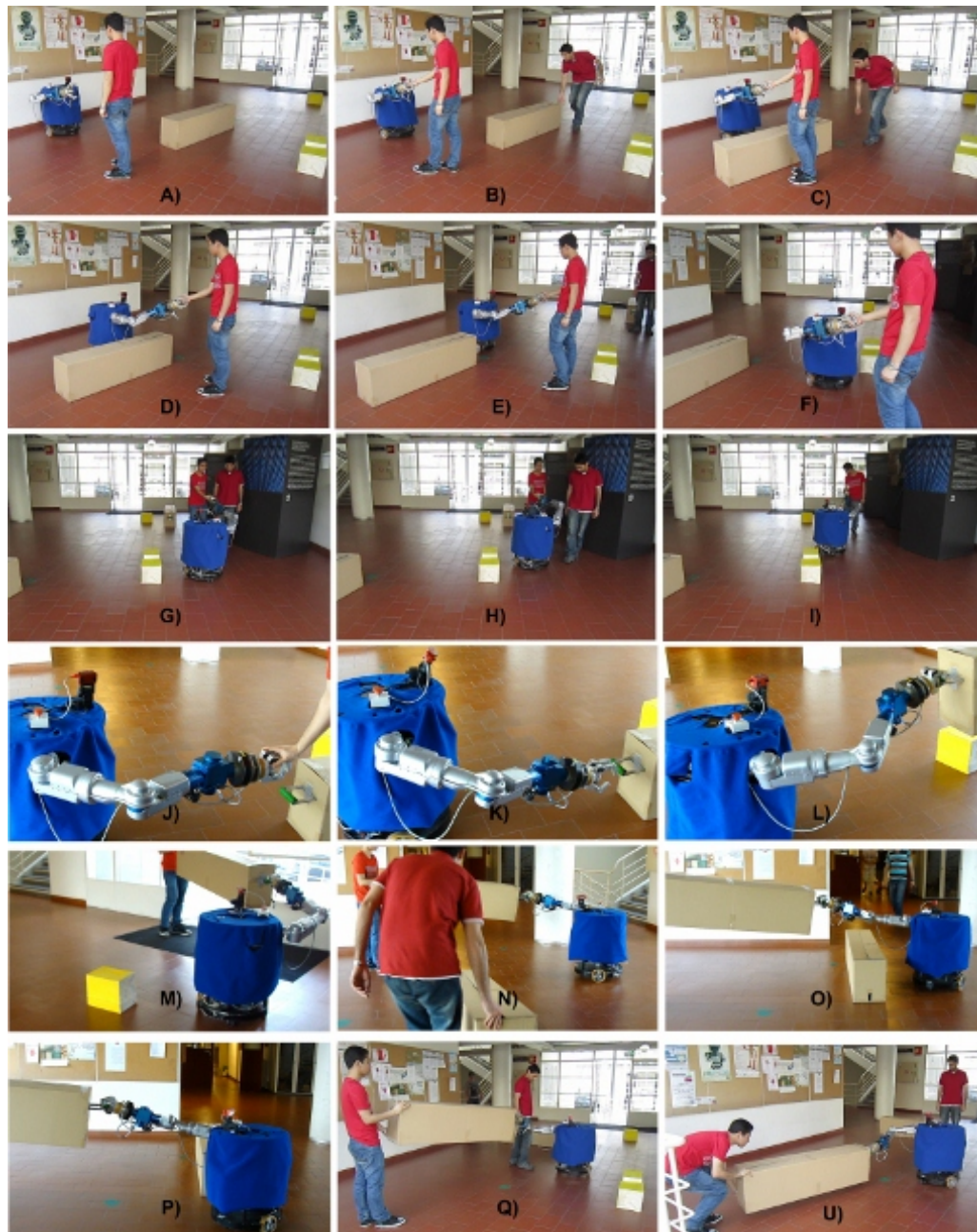
Figure 6.17: Scenario for illustrating the Human-Robot Joint Transportation task. A human partner holds the robotic hand and takes the robot to the object that he wants to transport (from A to I) with obstacles avoidance. After grasping the handle (J,K,L), the robot transports an object with a human partner in dynamic environment (from M to U) (Video 14).
