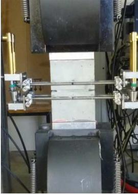
Figure 5: Tensile test setup for notched specimen
