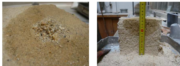
Figure 18 – Pitting depth and depth of moisture penetration.
