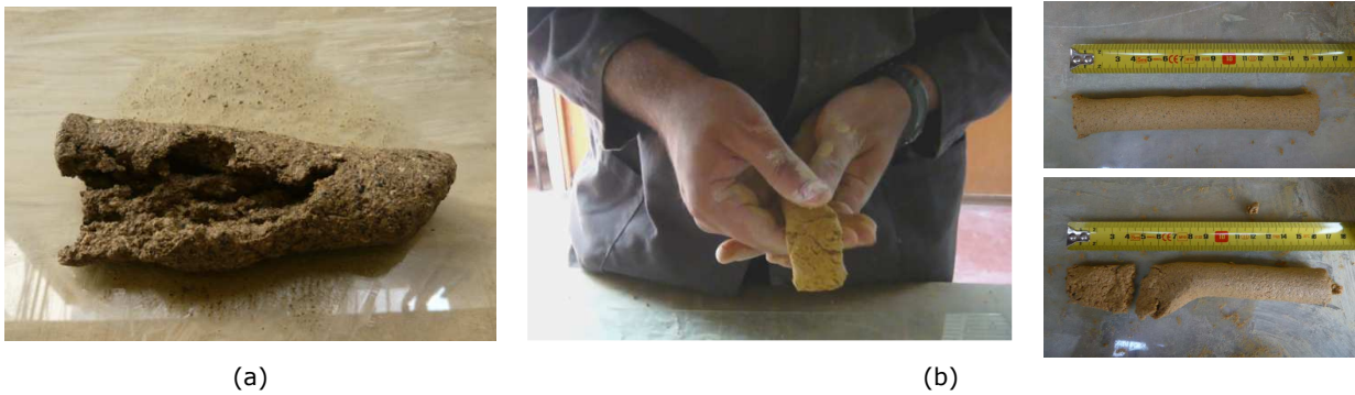
Figure 7 – Ribbon test of soil S1 (a) and ribbon test of soil S3 (b).
