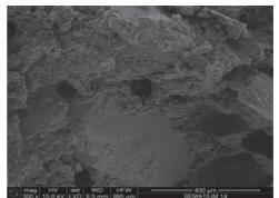
Fig. 5. Ordinary concrete at 28 days after casting
