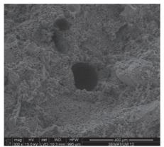
Fig. 8. Concrete with polyurethane at 28 days after casting
