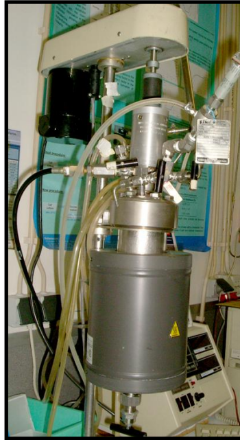
Figure 3.1 Stainless stirred bioreactor (PARR 4563, Parr Instruments, USA).
