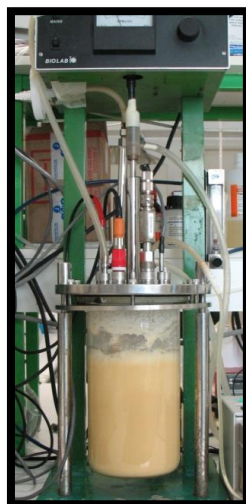
Figure 6.1 A 2-L bioreactor (BIOLAB, B. BRAUN, Germany) with P. pastoris culture growing in glycerol medium.
