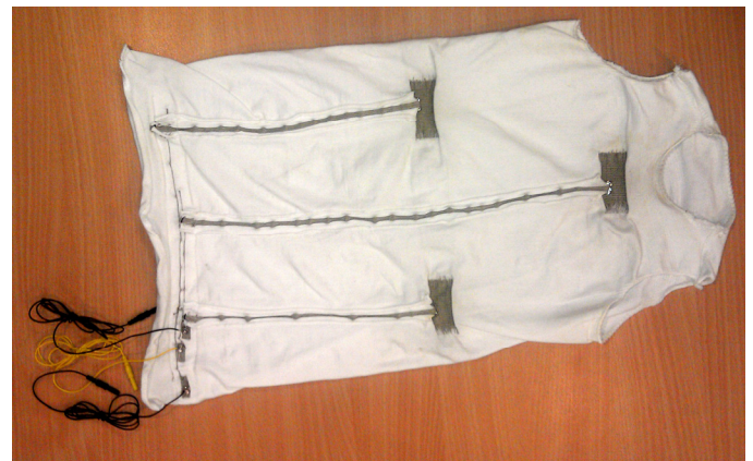
Fig. 5. Shirt with integrated textile electrodes
