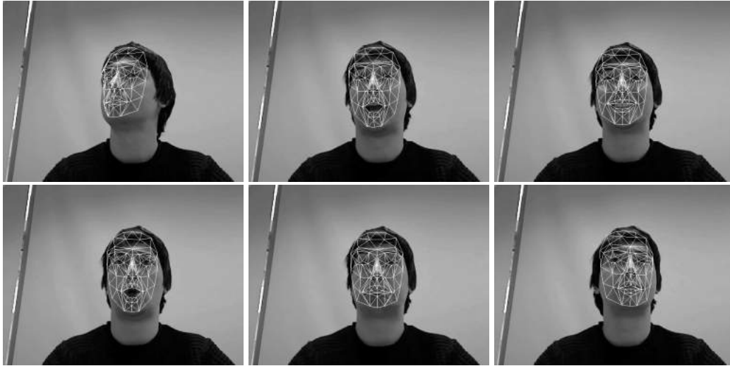
Figure 4: Images of the face model adjustment through OAM tracking [36] in a video, after applying the proposed initialization procedure in the first frame.
