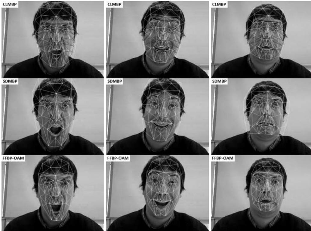
Figure 11: Comparison between CLMBP , SDMBP and FFBP-OAM in a video sequence with exaggerated facial expressions. The full sequence is available as supplementary material.
