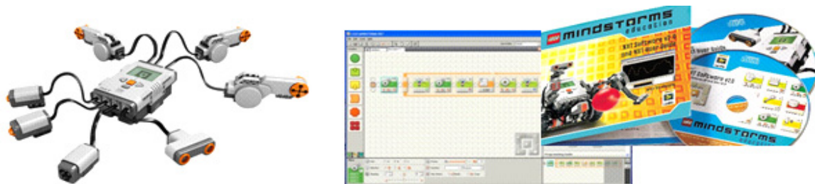
Figure 5: Lego® NXT controller with sensors and actuators (left) and programming resources (right).
