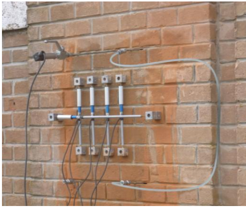
Figure 2. 20- Double flat jack test configuration on a brick masonry wall, Figure 2. 21- Stress strain diagram presenting results of double flat jack tests
