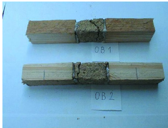
Figure 2. 17- Micro samples of mortar with wooden prosthesis
