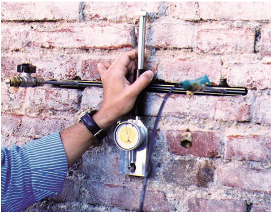
Figure 2. 18- Single flat jack inserted into cut, Figure 2. 19- Deformation stress diagram presenting results of single flat jack tests
