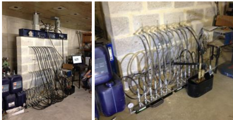
Figure 2. 22- tube jacks implicated on a masonry wall in laboratory at Minho University.
