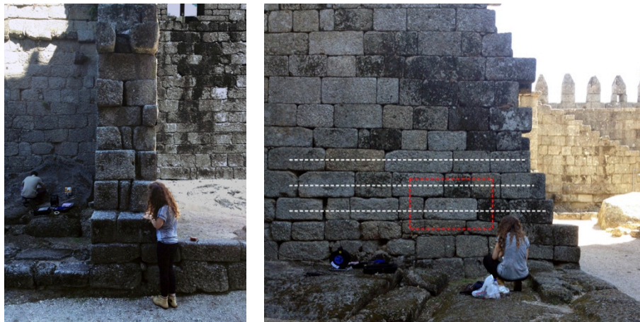
Figure 7. 4- Apparent section of the wall. Figure 7. 5- General layout of the tested wall (GPR profiles in with, sonic tested area in red)
