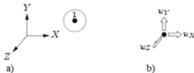
Figure 50 – Point mass: (a) Topology; (b) The three degrees of freedom (translations) of the PT3T element. [90]
