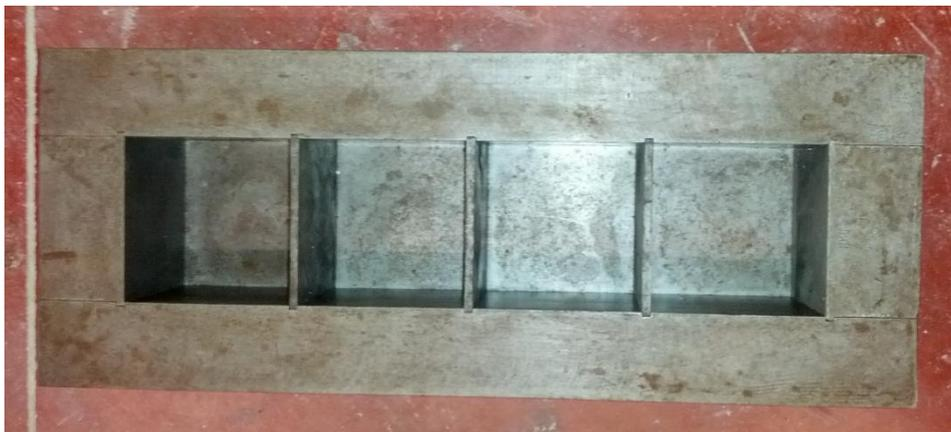
**Figura 3.10 – Moldes cúbicos ( $100 \times 100 \times 100$ ) ( $\text{mm}^3$ )**
