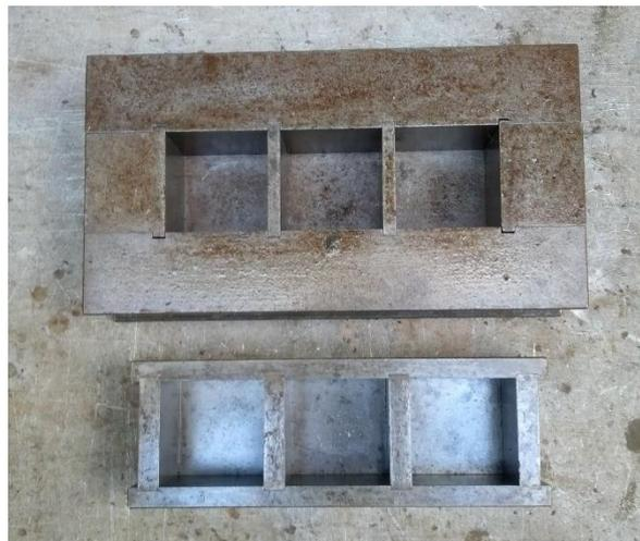
**Figura 3.9 - Moldes cúbicos ( $50 \times 50 \times 50$ ) ( $\text{mm}^3$ )**
