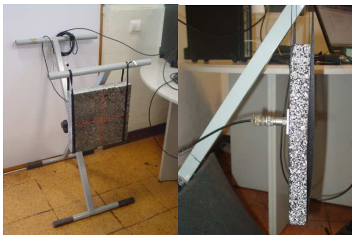
Figure 2 – Damping ratio testing set up
