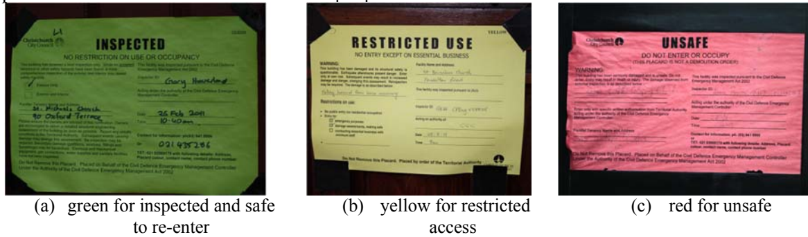
Figure 2. Placards given to buildings after Level 1 and Level 2 assessment.
