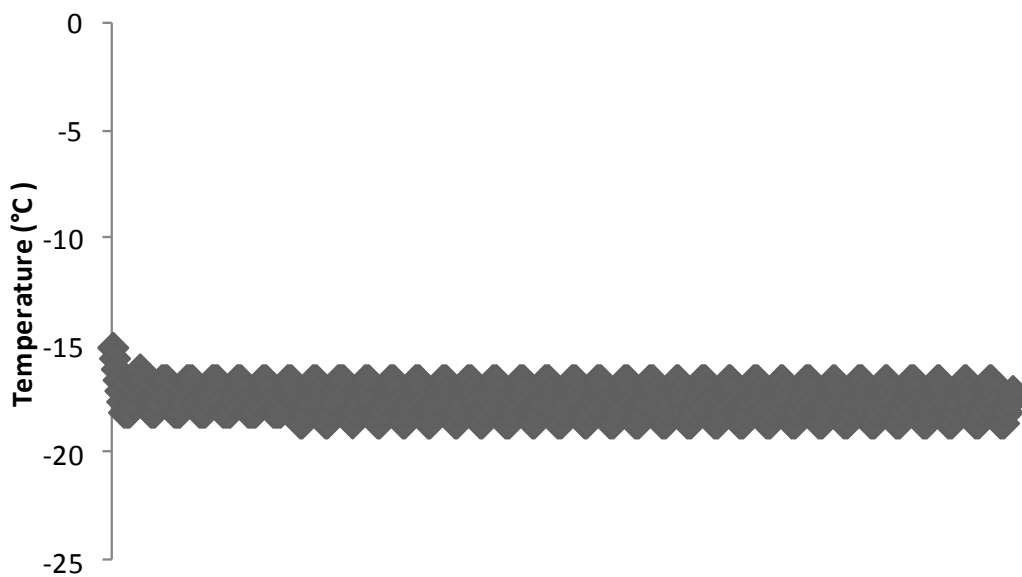
Figure A.15. Air temperature registered every 3 minutes of industrial freezing chamber programmed at -20 °C by a data logger during frozen storage
