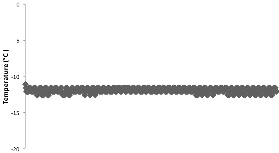
Figure A.14. Air temperature registered every 3 minutes of industrial freezing chamber programmed at -15 °C by a data logger during frozen storage
