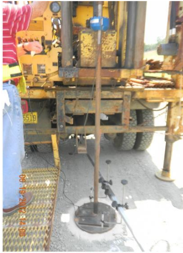
Figure 11 - Load Cell and Plate Set Up from NCDOT
