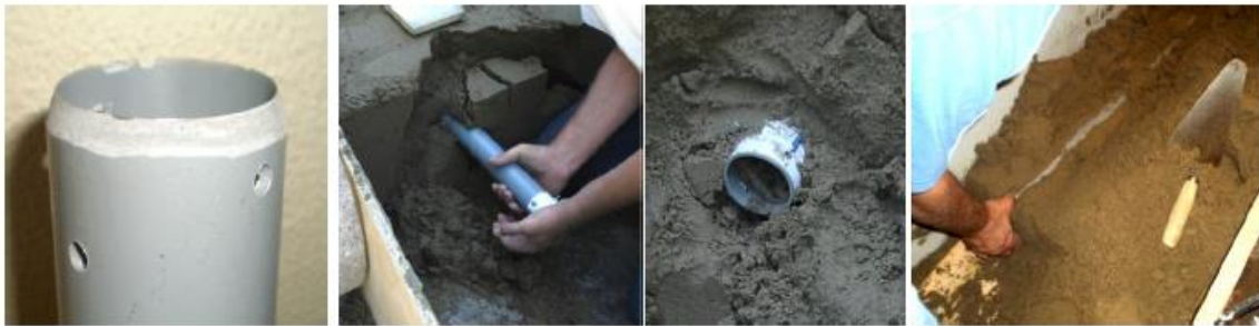
Figure 30 - Details of the sampling with the PVC tube (Costa 2011)
