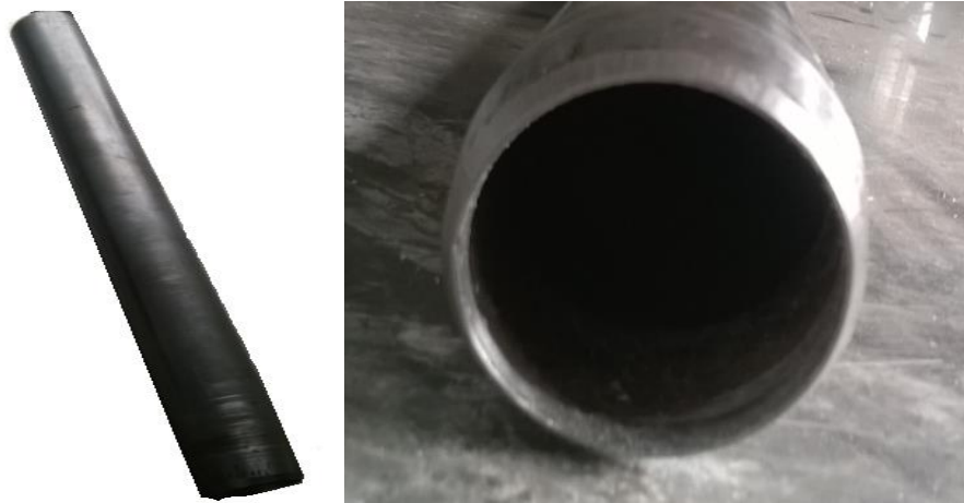
Figure 32 - Sampler and detail of the cutting edge
