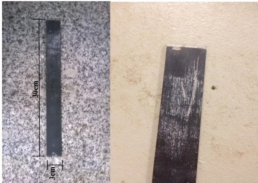
Figure 54 - Beam used and sharpened edge
