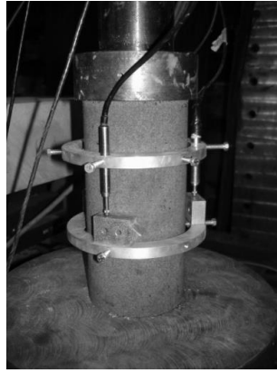
Figure 8 - Uniaxial compression test with LVDTs mounted (Silva 2010)
