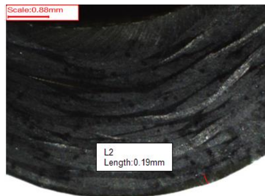
Figure 7. Resin excess measurements in point 2
