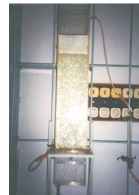
Fig. 1 - Rectangular bubble column
