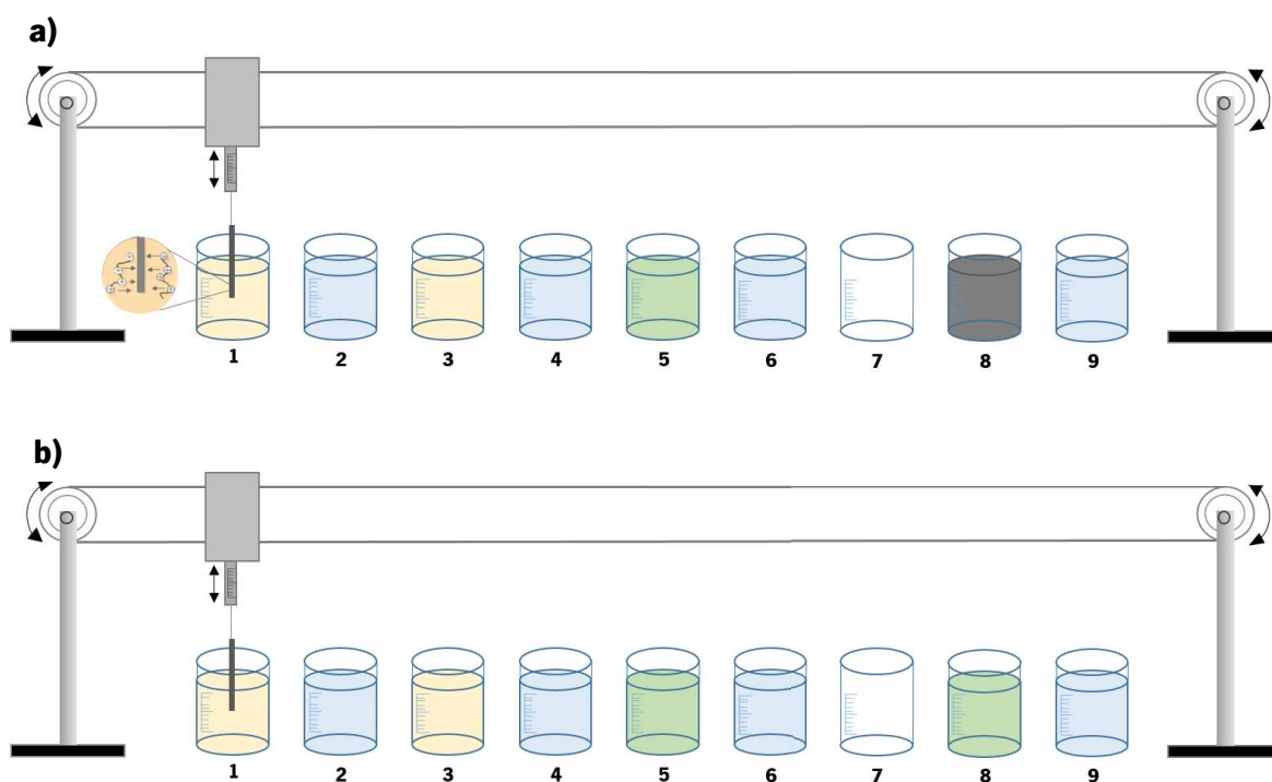
Figure 3.3 Schematic representation of the LbL processing. (a) Methodology used to produce (\text{CHI}/\text{ALG}/\text{CHI}/\text{o-GF})_{100} or (\text{CHI}/\text{ALG}/\text{CHI}/\text{o-GNR})_{100} where 1 and 5 : CHI solutions (2 mg/ml; pH=5.5); 2 , 4 and 6 : washing solutions (DW; pH=5.5); 3 : ALG solution (2 mg/ml; pH=5.5); 7 : empty cup; 8 : o-GF or o-GNR solutions (0.25 mg/ml; pH=8); 9 : washing solutions (DW; pH=8). (b) Methodology used to produce (\text{CHI}/\text{ALG}/\text{CHI}/\text{ALG})_{100} , where 1 and 5 : CHI solutions (2 mg/ml; pH=5.5); 2 , 4 and 6 : washing solutions (DW; pH=5.5); 3 : ALG solution (2 mg/ml; pH=5.5); 7 : empty cup; 8 : ALG solution (2 mg/ml; pH=5.5); 9 : washing solutions (DW; pH=5.5).
