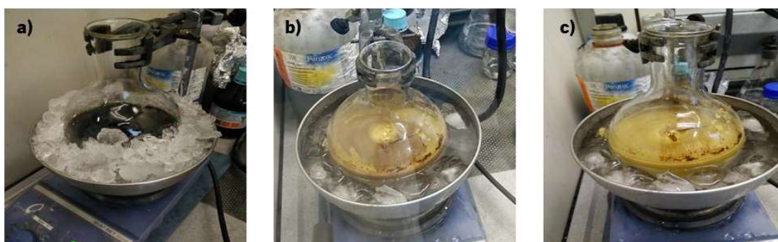
Figure 3.1 Representation of the color changing along with the procedure evolution. (a) Magnetic stirring of the solution with EG and \text{H}_2\text{SO}_4 (solution completely black); (b) solution after adding 300 mL of DW (brownish solution) and (c) solution following the \text{H}_2\text{O}_2 adding (yellow solution).
