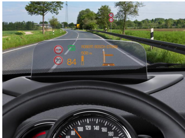
Figure 23 – Representation of Combiner Head-Up Display (Bosch Car Multimedia, 2014)
