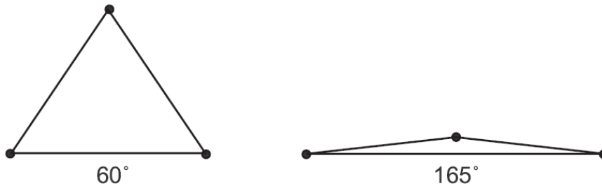
Figure 19 - Maximum Corner Angles for Triangles (ANSYS Inc., 2013)
