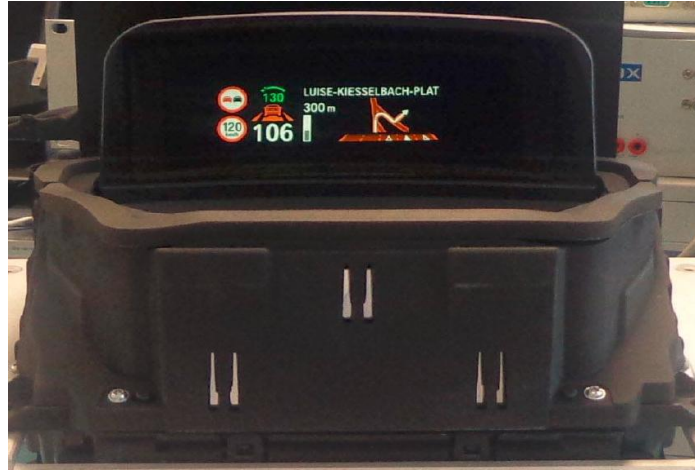
Figure 22 – Unit of Head-Up Display (Bosch Car Multimedia, 2014)
