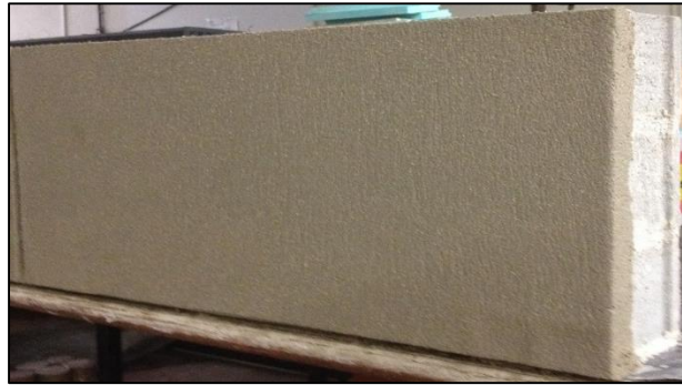
Figure 7.8. Structure reinforced masonry wall specimen.
