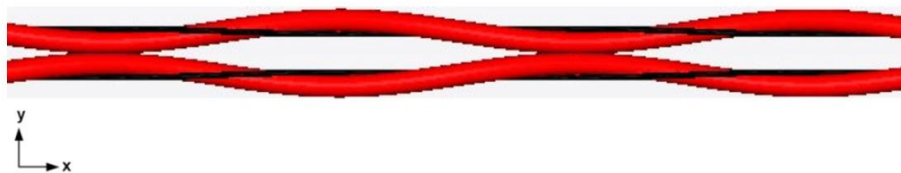
Figure 2.9. Textile application - pores open under tension in a complementary pair of HAYs [103, 104].
