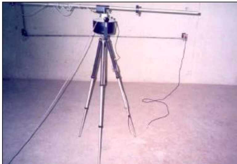
Figure 8: rotating microphone boom in the insulation chamber at the acoustic lab
