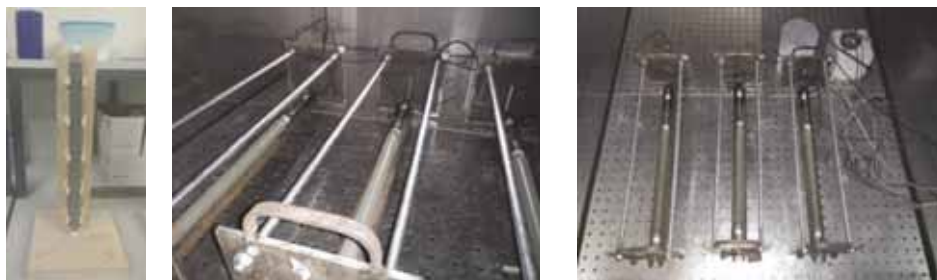
Figure 3 – Experimental setup for autogenous shrinkage testing.
