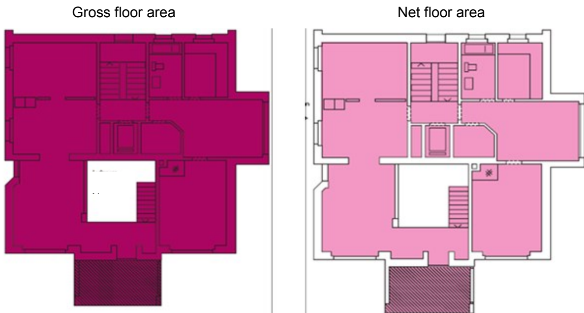
Figure 8 Illustration of (conditioned) gross floor area and net floor area. Hatched areas: Non conditioned exterior gross and net floor area respectively
