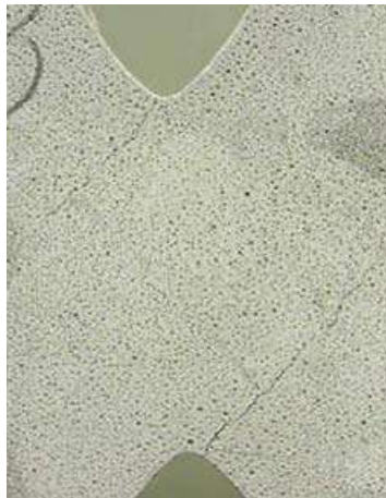
b) final crack pattern of PCM
