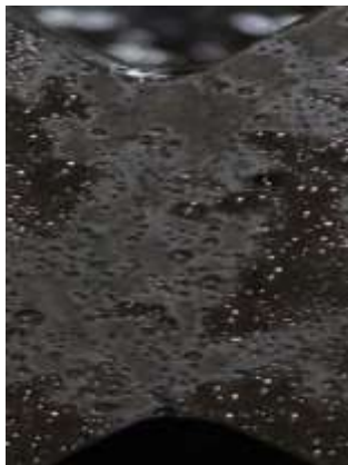
b) Crack pattern in the second phase (nonlinear pre-peak)
