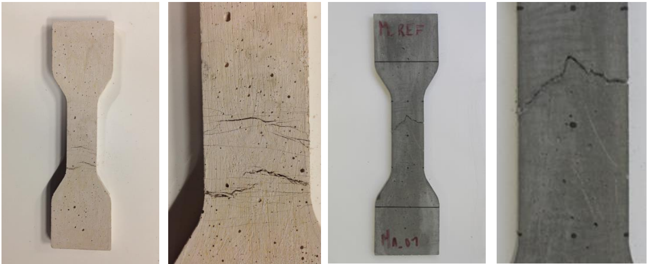
Fig. 4- Crack pattern of a geopolymeric and ECC specimen
