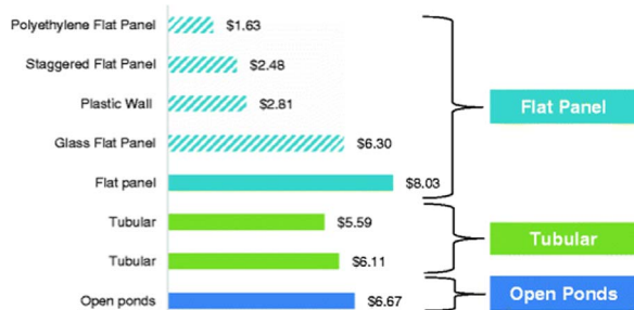
Fig. 11. Production cost in USD per kilogram calculated for the alkaline system and compared with values reported in literature for regular pH [137].
