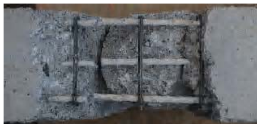
Figure 10 – Beam produced with braided reinforced composite rods after testing
