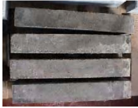
Figure 8 – Concrete beams reinforced by composite rods
