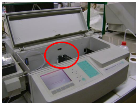
Fig. 1. Specimen inside the spectrophotometer.
