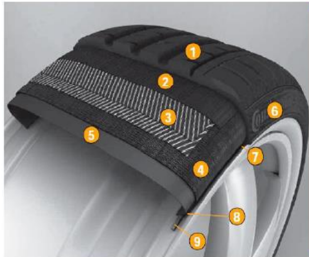
Figure 2- Cross section of a radial tire (adapted from [3])
