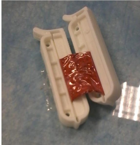
Figure 27 – SPATT made with dialysis bags.
